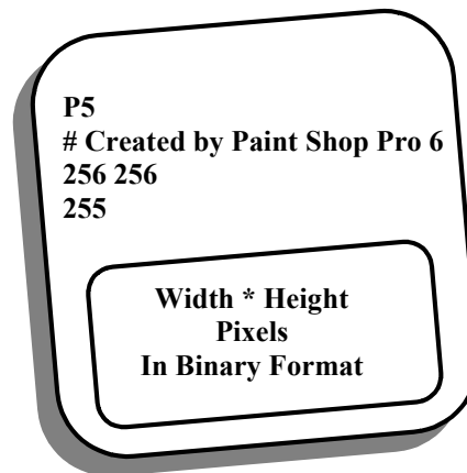
Fig. (2.1): Format Structure of PGM Image (Binary).
