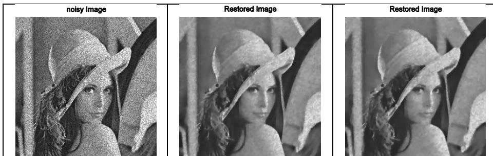
Fig. 7: (a) Problem.2 with variance \delta^2=0.03 (b) De-noised image by AA-model with number of iterations= 16. (c) De-noised image by ETMS with number of iteration=700. Choosing regularization parameters, \alpha_1 = 0.09 and \alpha_2 = 0.0003 .
