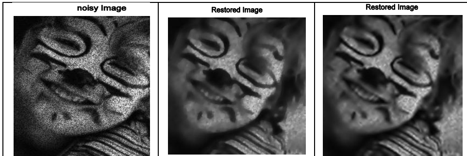
Fig. 2: (a) Problem.1 with variance \delta^2=0.1 (b) De-noised image by AA-model with number of iterations = 26. (c) De-noised image by ETMS with number of iteration=970. Choosing regularization parameters are \alpha_1 = 0.09 and \alpha_2 = 0.0003 .
