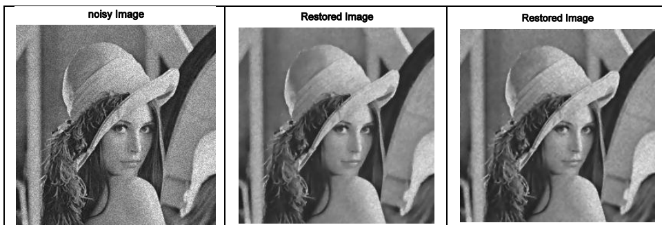
Fig. 6: (a) Problem.2 with variance \delta^2=0.01 (b) De-noised image by AA-model with number of iterations= 10. (c) De-noised image by ETMS with number of iteration=250. Choosing regularization parameters are \alpha_1 = 0.09 and \alpha_2 = 0.0003 .
