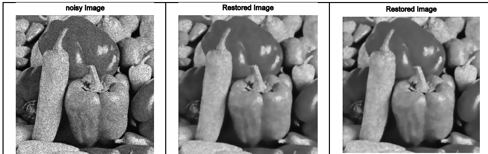
Fig. 10: (a) Problem.3 with variance \delta^2=0.03 (b) De-noised image by AA-model with number of iterations= 22. (c) De-noised image by ETMS with number of iteration=750. Choosing regularization parameters, \alpha_1 = 0.09 and \alpha_2 = 0.0003 .
