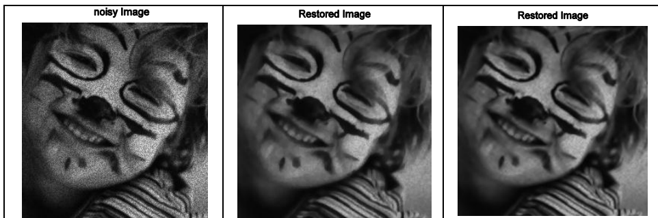
Fig. 3: (a) Problem.1 with variance \delta^2=0.01 (b) De-noised image by AA-model with number of iterations= 5. (c) De-noised image by ETMS with number of iteration=200. Choosing regularization parameters are \alpha_1 = 0.09 and \alpha_2 = 0.0003 .
